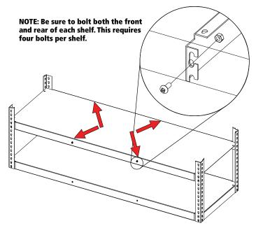
NOTE: Bolts are not needed to secure the deck supports on the bottom shelf because it rests on the floor. All other levels require these bolts to achieve maximum load capcities.
