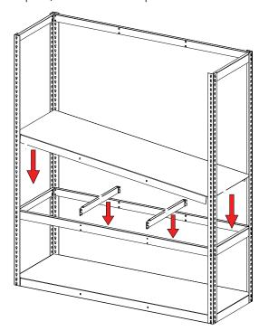
NOTE: Every fourth slot in the uprights has a flat top to help visually align the supports.
