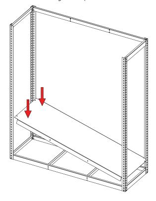
**5.** Attach shelf supports at the next desired shelf level. Once the shelf supports are in place, attach two front-to-back center supports as you did in step 3. Lower the steel decking into place, as described in step 4.
