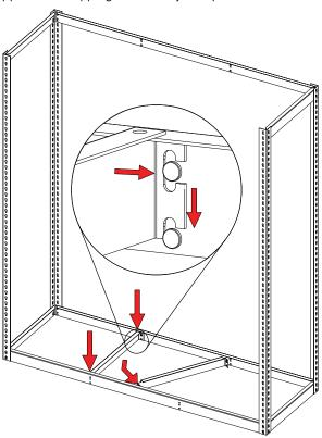
**4.** Lay the bottom decking (Ref. No. 5) on the shelf supports so that the front and back edges overlap the front and back shelf supports.
